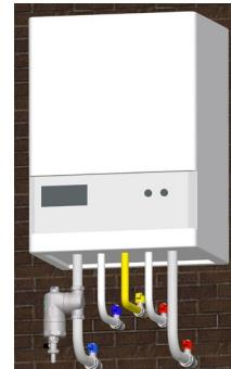
The figure shows a dirt separator installed on the return line with the swivelling connection in vertical position. This configuration is recommended when you have space vertically below the boiler.
